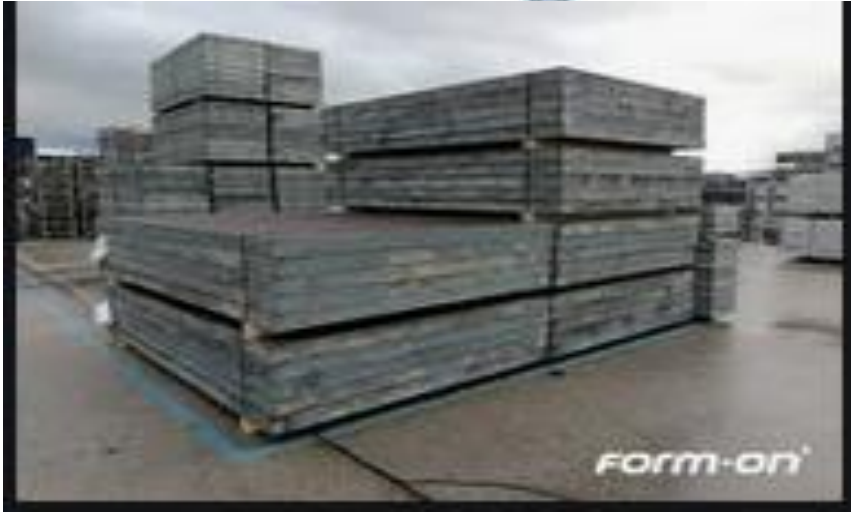
Fig 5. Steel formwork storage
